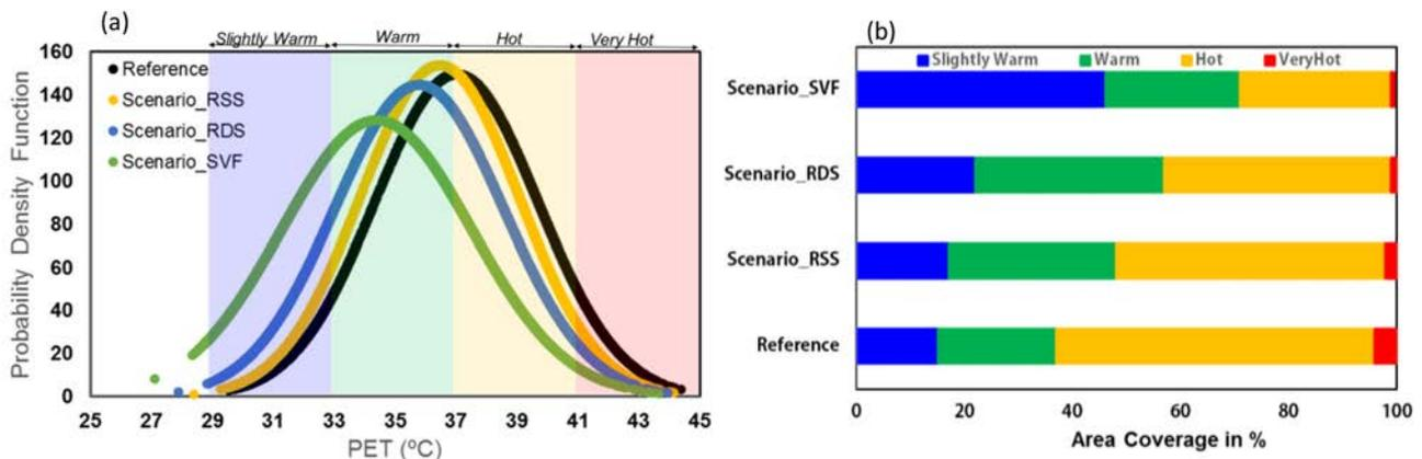
Fig. 14. (a) Probability density distribution of domain and time-averaged PET values for all scenarios (b) Area coverage of thermal forms in different scenarios on at pedestrian level.
