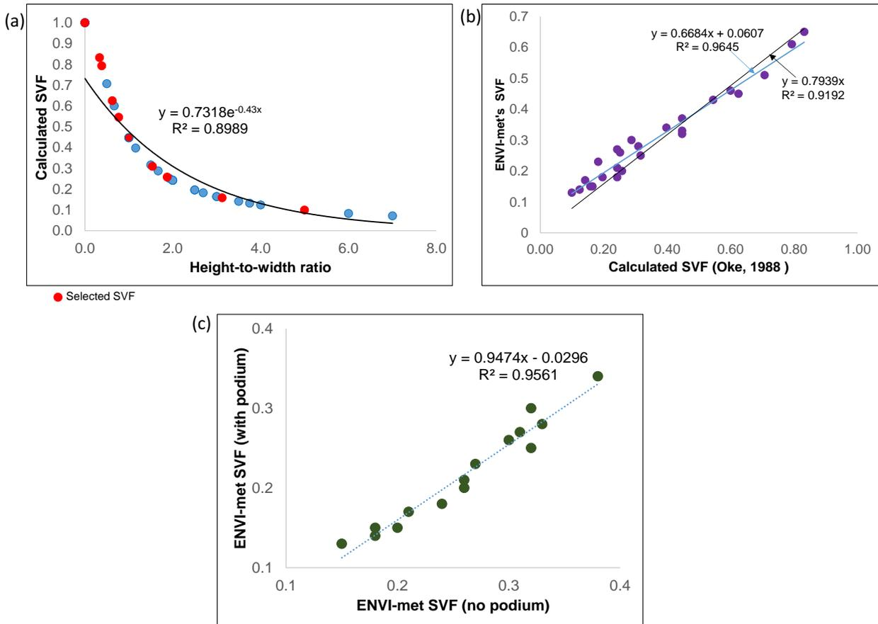
Fig. 4. (a) Relationship between aspect ratio and sky-view factor (b) Relationship between ENVI-met and Oke’s method of SVF calculation (c) Comparing SVF in street canyons of bounding buildings with and without a podium.
