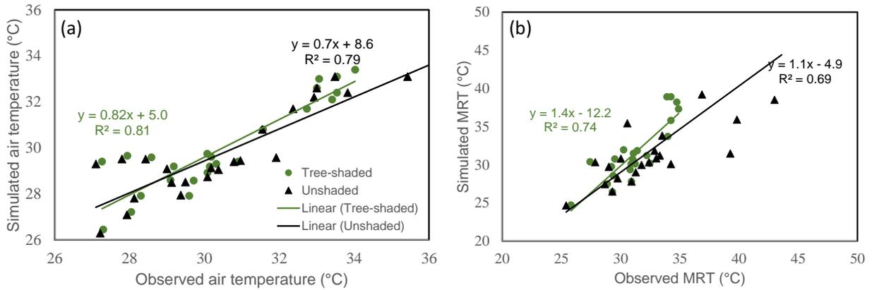
Fig. A1. Relationship between ENVI-met simulated and observed (a) air temperature and (b) mean radiant temperature, MRT at tree-shaded and unshaded location on 23rd August, 15th and 17th October 2016 (09:00–17:00 local time) (source: (Morakinyo et al., 2018)).
