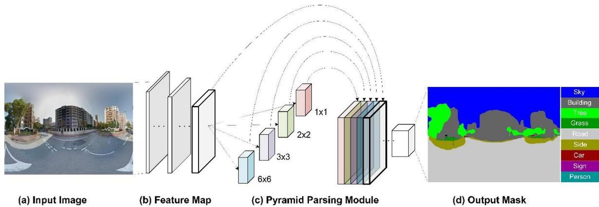
**Fig. 2.** Workflow of semantic scene parsing using PSPNet. For a given input street view image in **(a)**, the network extracts the feature map in **(b)**, and then the pyramid parsing module is applied to form the final feature representation of the streetscape in **(c)**. Finally, a pixel-wise classified output street view image with semantic categories in **(d)** is produced by feeding the feature representation into a convolution layer.
