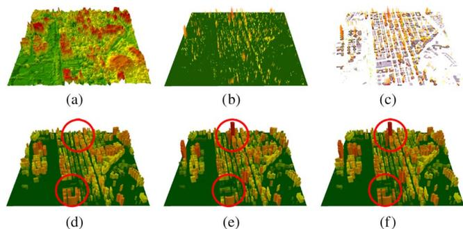
Fig. 3. Building height retrieval using different approaches. (a) Initial height result using stereo images (unit: meters). (b) Initial height result using SAR images (unit: meters). (c) Prior building footprints, in which matched buildings are marked with black color, whereas matched SAR objects are marked with red color. (d) Result using the stereo images. (e) Result using the SAR images. (f) Result using the fusion approach.
