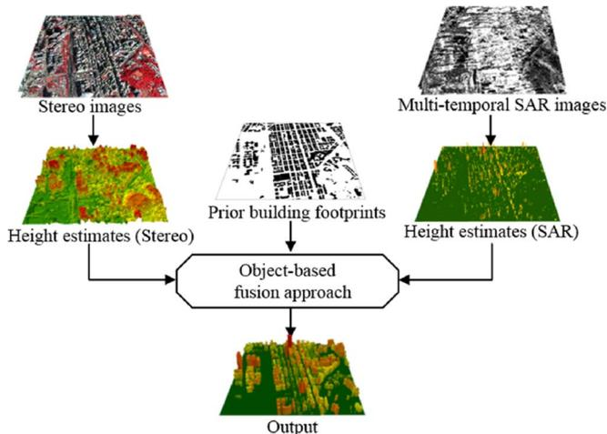
Fig. 1. Procedure of the proposed approach for building height retrieval.
