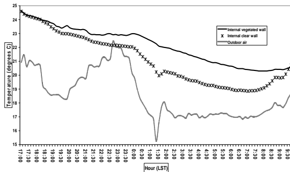
Fig 8. Comparison of internal air temperatures for the vegetated and clear walls at 9-10-03.
