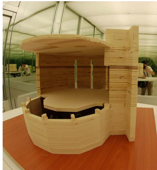
Fig 13. Daylight model inside the artificial sky (scale 1:30)
