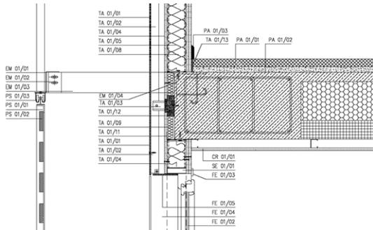
Fig 3. Detail of the light-weight façade with the thermal bridges treated in the intersections with the structure and with sliding solar protections of windows.
