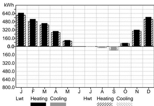
Fig 4. Lwt vs Hwt. Monthly heating and cooling loads of the flat PISO\_A.
