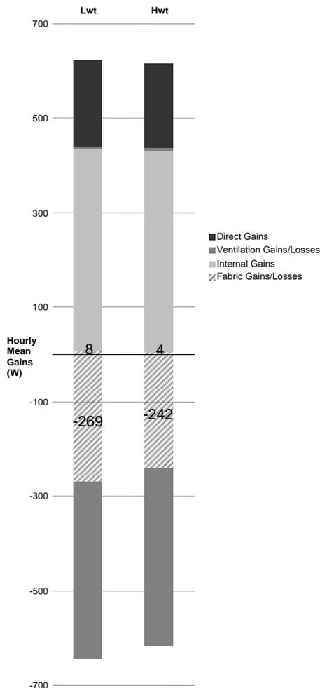
Fig 6. Load distribution in Lwt and Hwt options.
