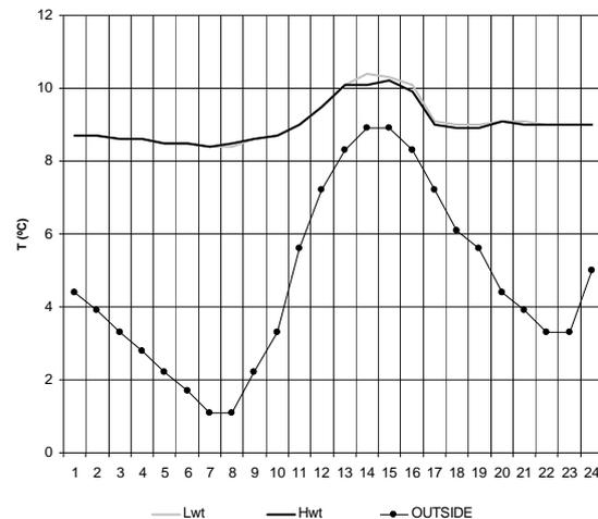
Fig 8. Lwt and Hwt Hourly temperature of the Coldest Peak Day
