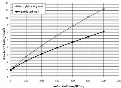
Fig 6. Wall heat gain. Ventilated vs. sealed cavity. Winter case
