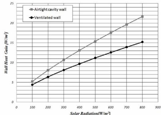
Fig 6. Wall heat gain. Ventilated vs. sealed cavity. Summer case
