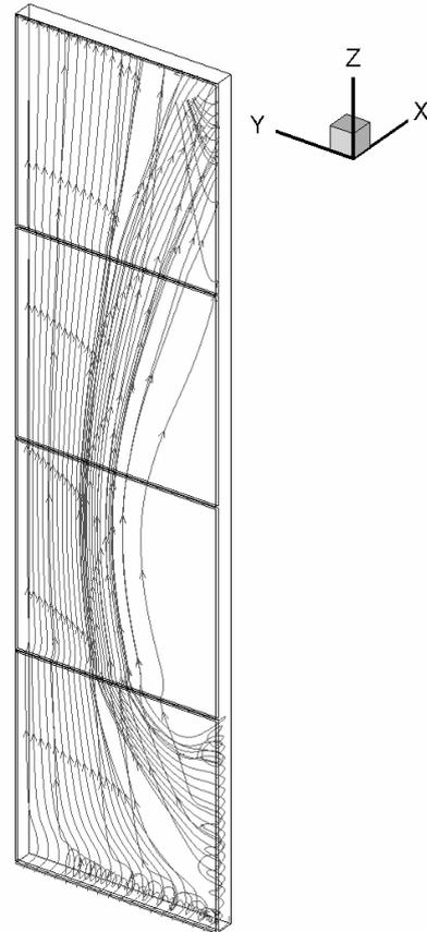
Fig 6. Streamlines of air moving along the cavity
