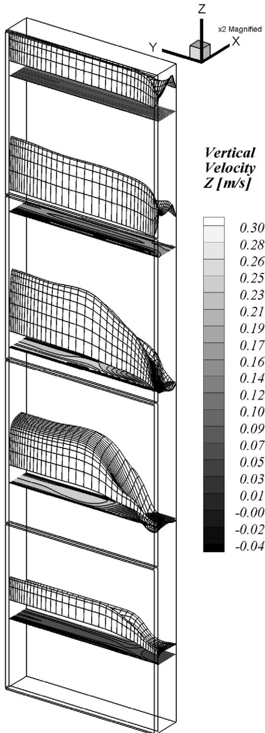
Fig 5. Z-velocity profiles inside the ventilated wall
