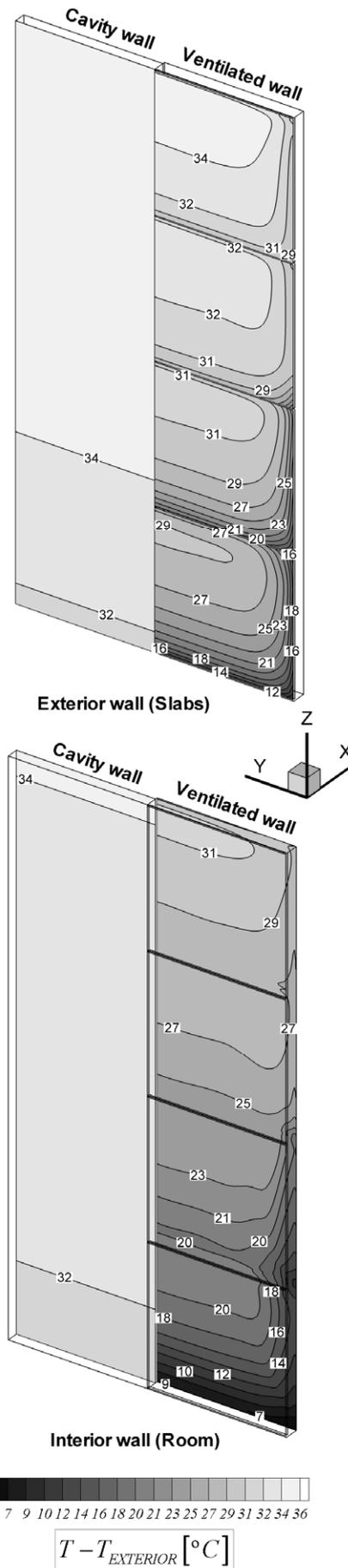
Fig 4. Comparison of temperature rises over ambient
