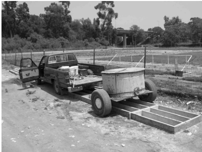
Image 3. Papercrete tow mixer and block forms.
