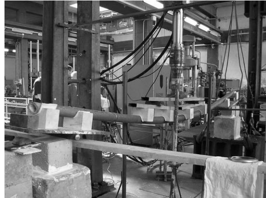
Fig 7. Physical resistance test of a bamboo culm held at the Polytechnic of Turin in 2007.
