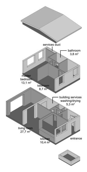
Fig 4. Improved layout, small type of dwelling Walls and roofs to be added are shown in a darker grey
