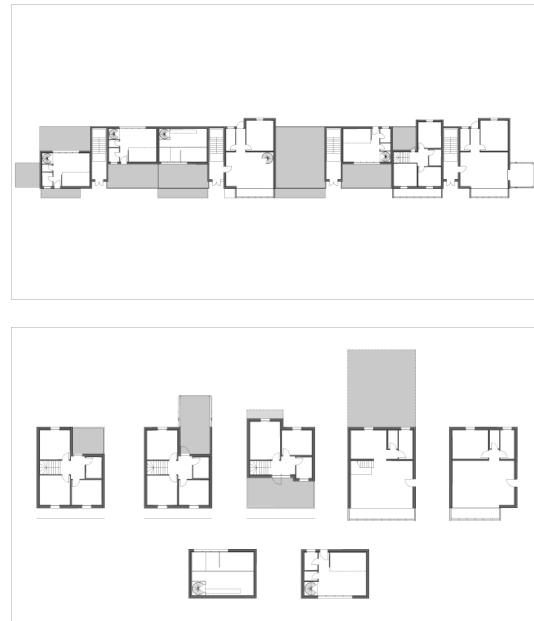
Fig 5. TOP: one of the possible configurations of a block of flats. A private open space is attached to each unit. BELOW: Some of the possible configurations of single dwelling.
