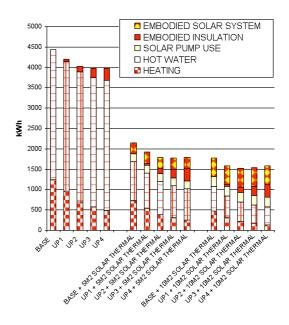
Figure 4. Annual space & water heating embodied energy for insulation and solar systems, and electricity use for the solar pump.
