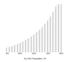
Fig 2. Temperature lines – the psychrometric chart
