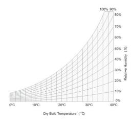
Fig 4. Psychrometric chart - showing lines of temperature and relative humidity
