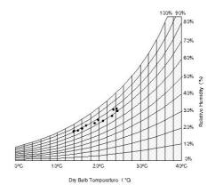
Fig 7. Example given for climate classification and for design purposes – Porto Alegre's climate data plotted in the psychrometric chart
