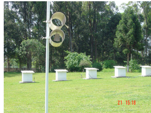
Figure 2: Set-up: Ambient temperature measurements and set of test cells.
