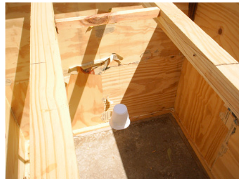
Figure 3: Internal temperature measurements with HOBO logger enclosed in a plastic cup.
