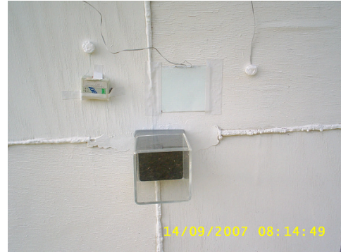
Figure 1: Set-up: HOBO data logger, Heat flux plate, thermocouples and solarimeter.
