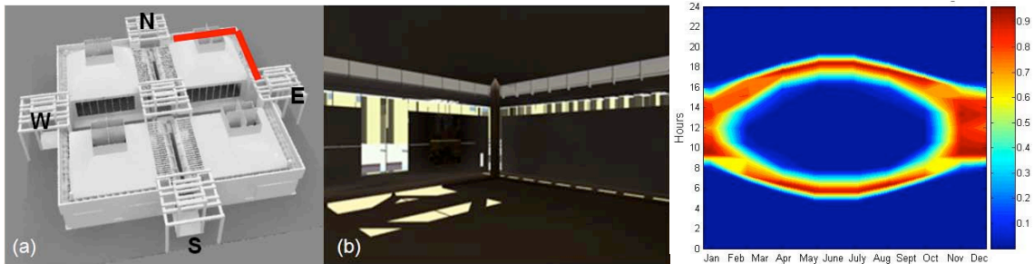
Figure 3. Renderings of a museum case study in Boston: (a) Radiance model - the considered areas are indicated for the NE exhibit space; (b) Interior rendering (3ds Max® by Autodesk®) on May 29 at noon; (c) time-varied performance.
