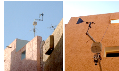
Figure 4 : Two examples of measuring stations localization. At left, measurements taken above the roof. At right, measurements taken within street.
