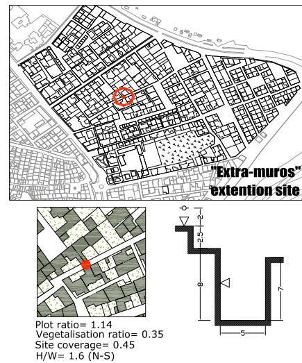
Figure 7: “Extra muros” extension measurement point.
