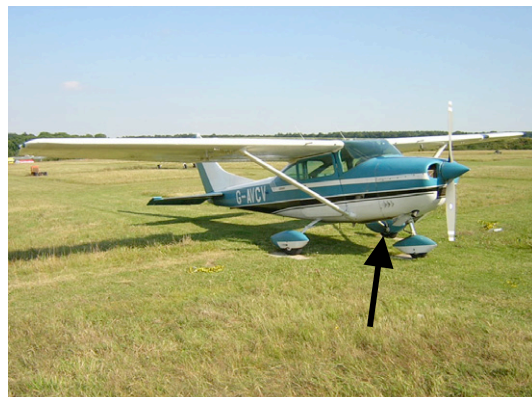
Fig 4. Cessna-182J carrying KT19 sensor, which records temperature and humidity (arrowed)
