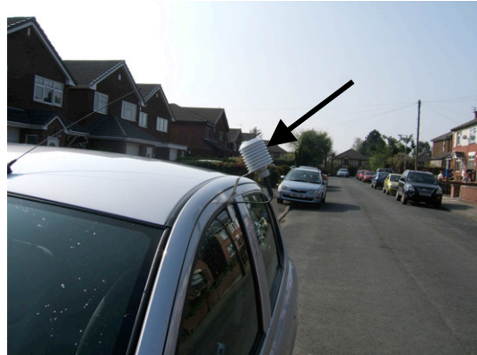
Fig 3. Car fitted with Rotronic AG HygrologNT sensor (arrowed), which records temperature and humidity
