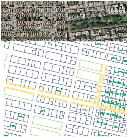
Fig 3. Top: Aerial shots of a typical urban environment. Bottom: Typical urban scene with different regions (orange: avenue zone, green: block zone, dark green: patio zones, blue: lot zones).
