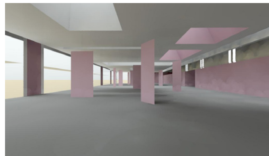
Fig 7. Placement of skylights above the reading areas.
