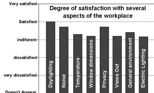
Fig 7. Occupants' degree of satisfaction with their indoor environment (results from a formal written survey issued to 90 occupants of the building)
