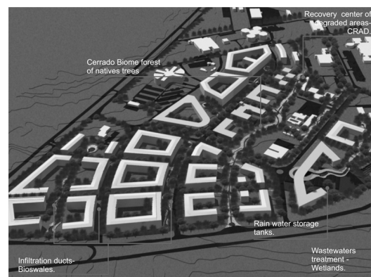
Fig 1 – Green infrastructure techniques applied to the urban design: bioswales, green fences, storage tanks and residual water treatment.
