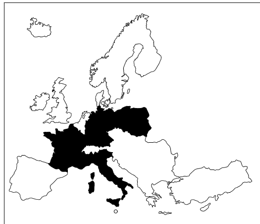
Fig 4: Area required replacing natural gas consumption of Europe by 1 st generation biomass; here rapeseed as energy crop. Calculations based on [1] and [3]
