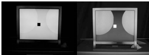
Fig 6. A type I glossy screen with calculated high L_{max} but still presents distracting reflections.
