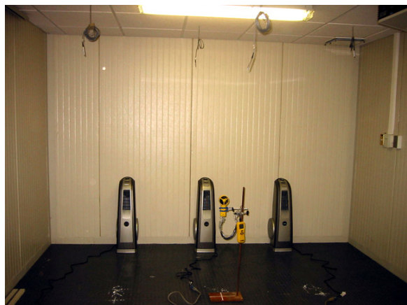
Figure 3: Laboratory of Controlled Ambient Conditions Calibration of fans used in the experiment
