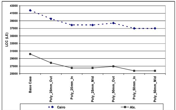
Studying LCC and the impact of wall insulation on energy consumption shows that the optimum wall insulation is 25 mm polystyrene mid
