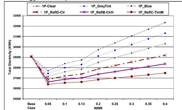
The simulation shows the optimum WWR is .15 with 1P ref B-clr H in Alex.
