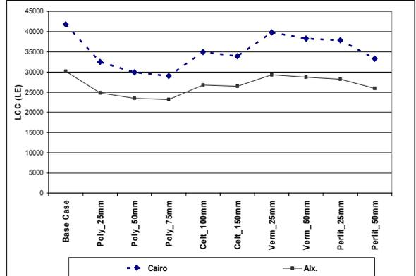
Studying LCC and the impact of roof insulation on energy consumption shows that the optimum roof insulation is 50 mm polystyrene or 150 mm siliton
