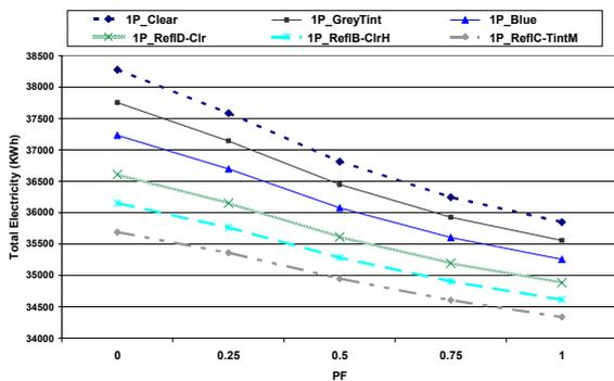
**Figure 6:** Impact of projection factor and SHGC on life cycle cost (LCC) in Cairo
