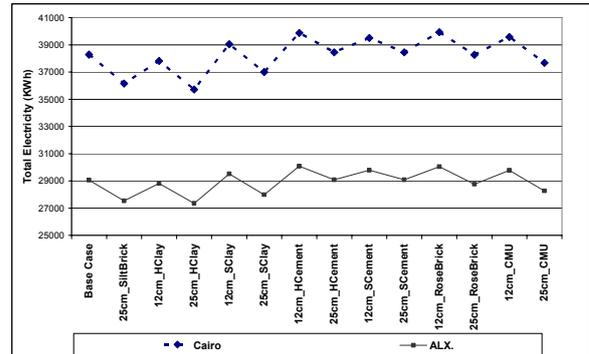
The simulation shows that using 25 cm of wall construction is better than 12 cm and using silt or
