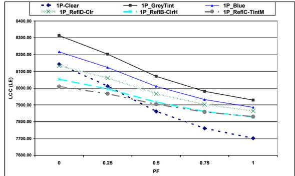
Studying LCC and the impact of projection factor and SHGC on energy consumption in Cairo shows That the optimum PF is 0.5m with 1P ref B-clr H or 1P ref C-Tint M
