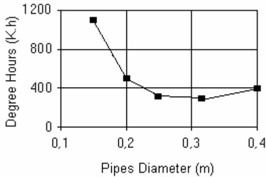
**Figure 5:** Number of cooling degree hours as a function of the diameter of the pipes.
