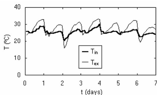
**Figure 3:** Outdoor air temperature ( $T_{ex}$ ) and predicted indoor air temperature with the passive cooling system ( $T_{in}$ ).
