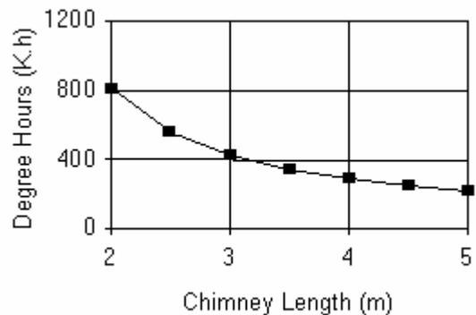
**Figure 8:** Number of cooling degree hours as a function of the length of the chimney.
