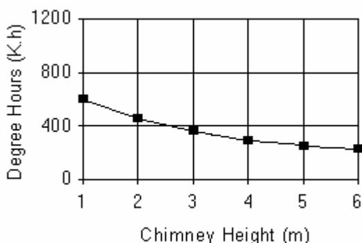
**Figure 9:** Number of cooling degree hours in function of the height of the chimney.
