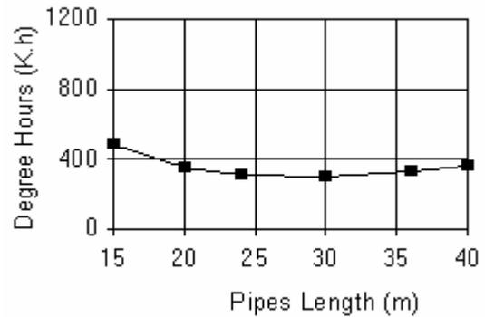
**Figure 7:** Number of cooling degree hours in function of the length of the pipes.
