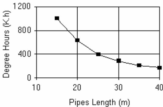
**Figure 6:** Number of cooling degree hours in function of the length of the pipes.
