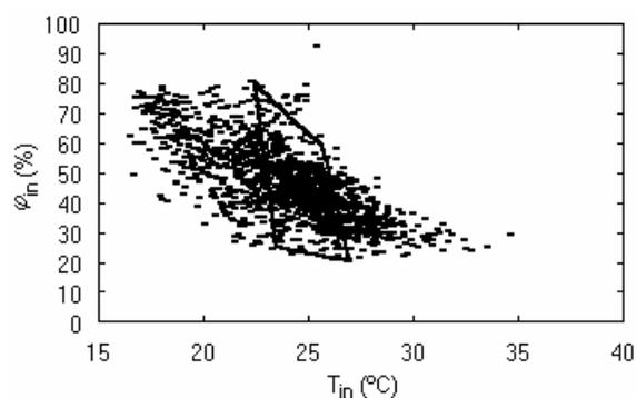
**Figure 2:** Thermal environment, inside the office with solar chimney and buried pipes
