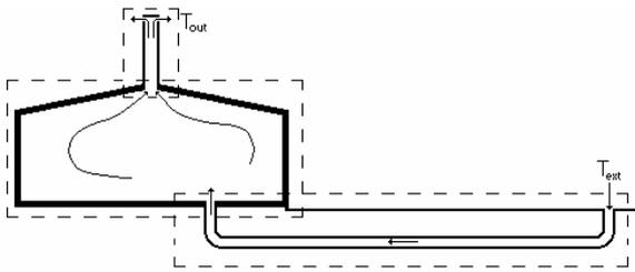
Figure 1: Building, solar chimney and buried pipes
