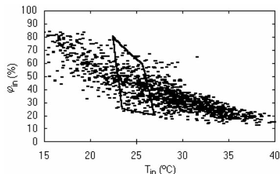
**Figure 4:** Thermal environment within the office with solar chimney and without buried pipes.
