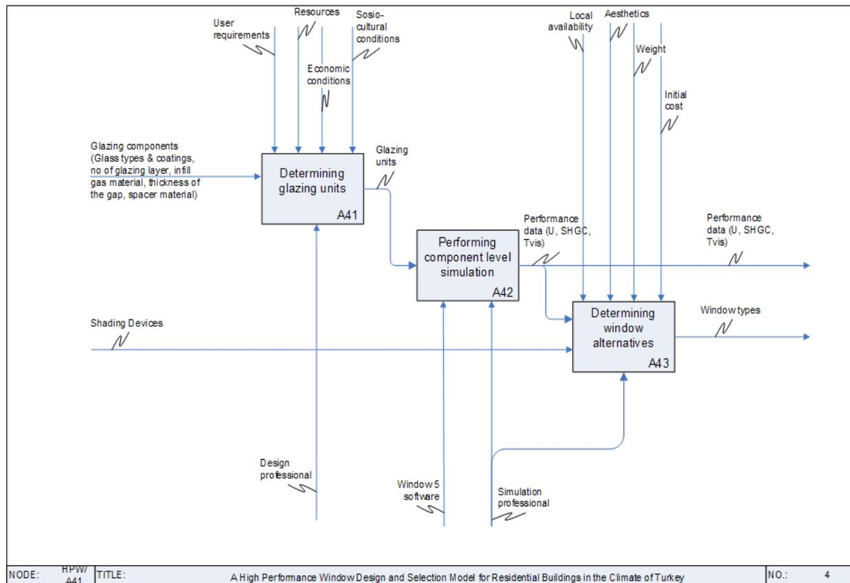
**Figure 3:** The inputs, outputs, controls and mechanisms of developing window system alternatives
