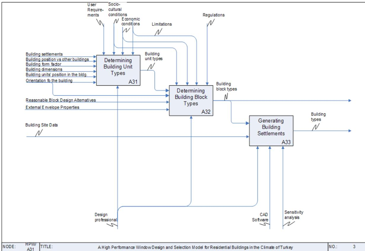
Figure 2: The inputs, outputs, controls and mechanisms of designing the typical residential buildings
