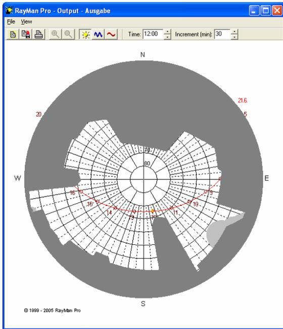
Figure 6: Output of sun path and horizon limitation.
