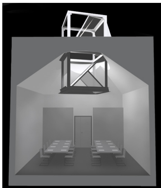
Figure 15: Venice 21 February at 9.00 a.m. Internal luminance distribution with skylight incorporating heliostat / proposed device
