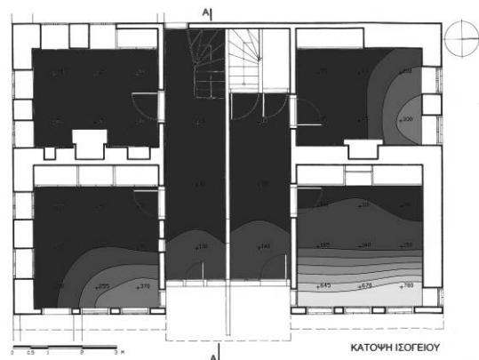
Figure 11: Ground floor. Daylighting measurements at 12:00 TST.
