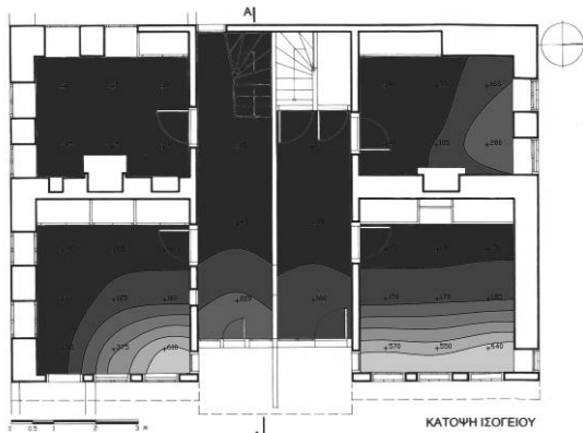
Figure 12: Ground floor. Daylighting measurements at 15:00 TST.
