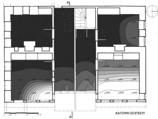
Figure 10: Ground floor. Daylighting measurements at 09:00 TST.
