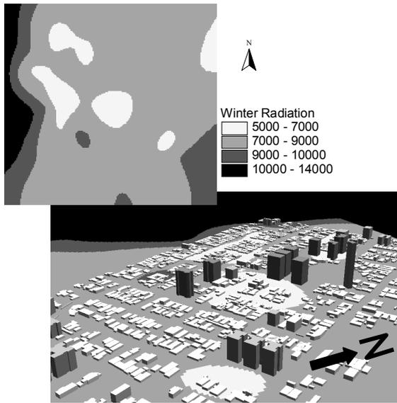
**Figure 7:** Radiation on a horizontal surface expressed in  $\text{Wh/m}^2$  during winter solstice.
