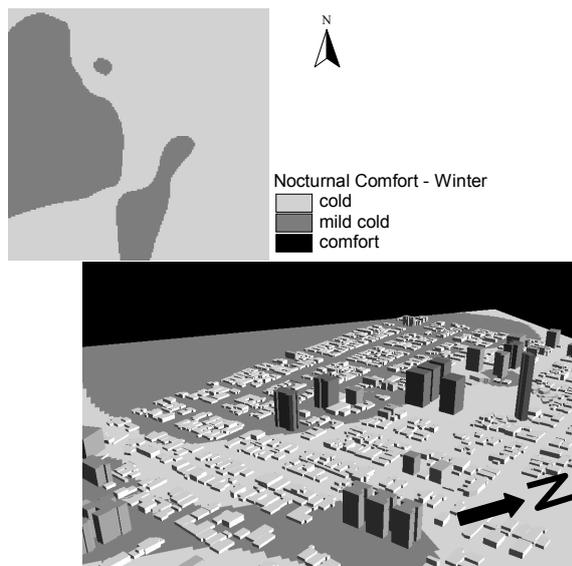
**Figure 13:** Nocturnal comfort in winter, considering the Mahoney nocturnal range of 17 to 21 °C. The semantic scale means: cold from 12 to 14°C; mild cold from 14 to 17°C – results are based on the minimum temperature analysis.
