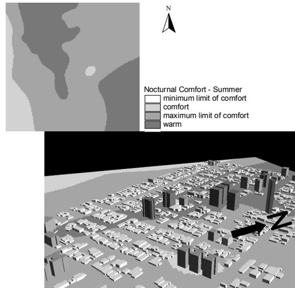
**Figure 11:** Nocturnal comfort in summer, considering the Mahoney nocturnal comfort range of 17 to 21°C. The semantic scale means: mild cold from 15 to 17°C; warm from 21 to 25°C – results are based on the minimum temperature analysis.
