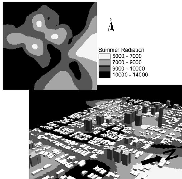
**Figure 6:** Radiation on a horizontal surface expressed in  $\text{Wh/m}^2$  during summer solstice.
