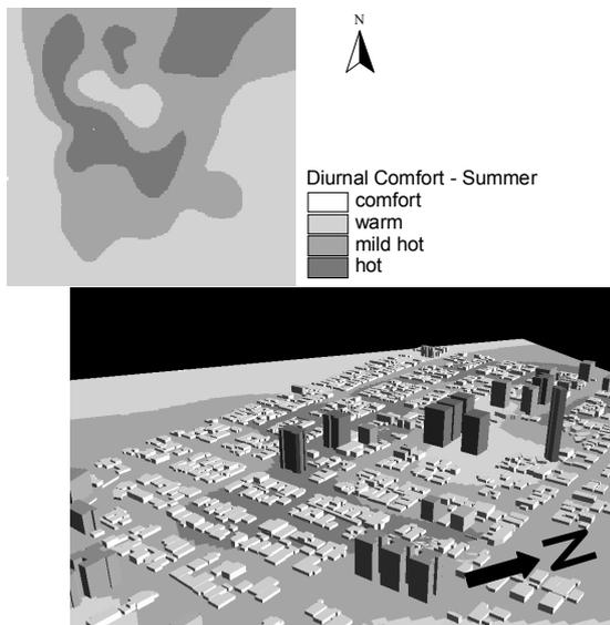
**Figure 10:** Diurnal comfort in summer, considering the Mahoney diurnal comfort range of 22 to 27°C. The semantic scale means: warm from 28 to 30°C; mild hot from 30 to 32°C; hot from 32 to 35°C. Results are based on the maximum temperature analysis.
