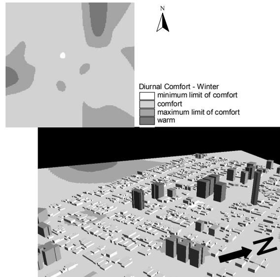
**Figure 12:** Diurnal comfort in winter, considering the Mahoney diurnal range of 23 to 29°C. The semantic scale means: mild cold from 21 to 23°C; warm from 29 to 30°C – results are based on the maximum temperature analysis.
