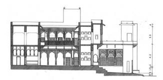
Figure 8: Longitudinal Section Through Both Courtyards
