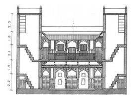
Figure 7: Transverse Section Through Internal courtyard
