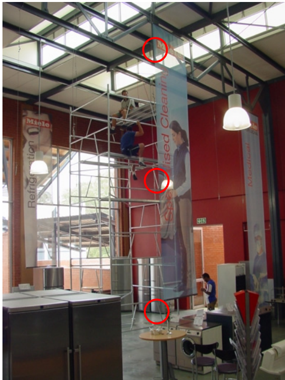
Figure 9: Chains suspended from underside of truss and showing positions of thermometers
