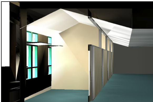
Figure 5: Rendering of office with light shelf
