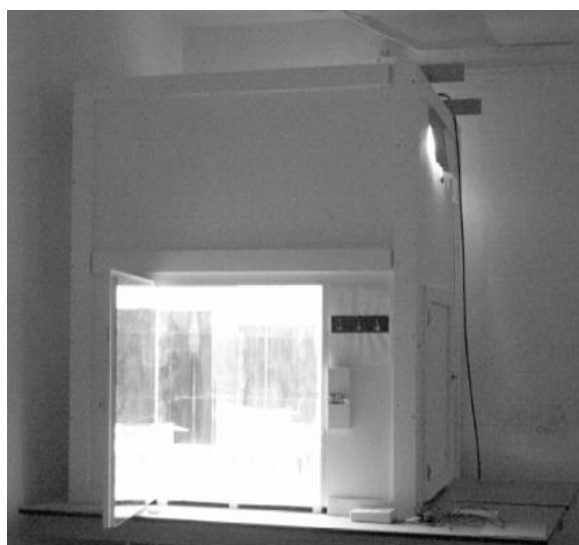
Figure 3: Artificial sky (overcast) at Laval University's School of Architecture, Québec, Canada, used for physical model studies.
