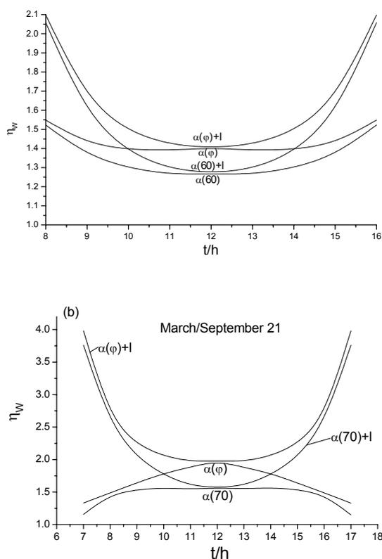
**Figure 4:** The dependence of the irradiance enhancement coefficient on time, on the shortest day of the year (a) and on the equinoxes (b), at 44° NL in a greenhouse with reflecting walls inclined at optimum angles,  $\alpha(60)$  and  $\alpha(70)$ , as well as with those of changing inclination.
