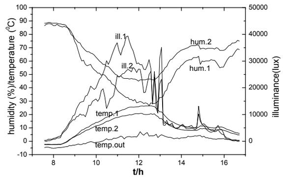
**Figure 9:** Experimental measurements of illuminance, temperature and humidity in the greenhouse with a reflecting wall with the inclination fixed at 70°, without the use of louvres, compared to those taken in the control-greenhouse.
