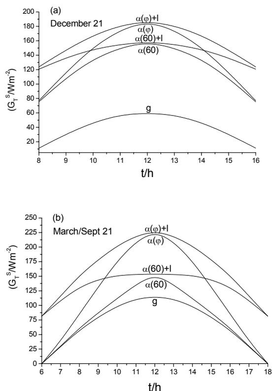
**Figure 3:** Calculated dependence of the ground irradiance on time for the shortest day of the year (a) and for the equinoxes (b) in a greenhouse without (g) and with a reflecting wall inclined at an angle of  $60^\circ$ , ( $\alpha(60)$ ), as well as with that of changing inclination, ( $\alpha(\phi)$ ), without louvres and the same with louvres ( $\alpha(60) + I$  and  $\alpha(\phi) + I$ ).
