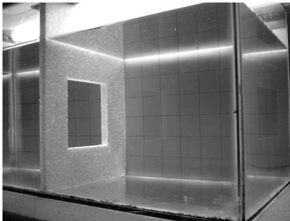
Figure 5: Scaled immersion model of the room with single opening.
