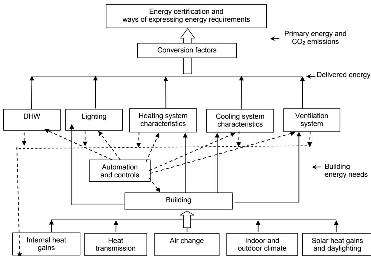
**Figure 2:** Energy flows and their links. The bottom row indicates the input data, comprising the building characteristics, its usage and climatic parameters. Recovered losses from systems contribute to the heat gains.
