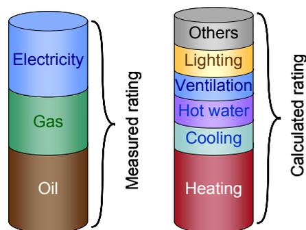
**Figure 3:** The two types of energy ratings proposed in prEN 15203/15315.
