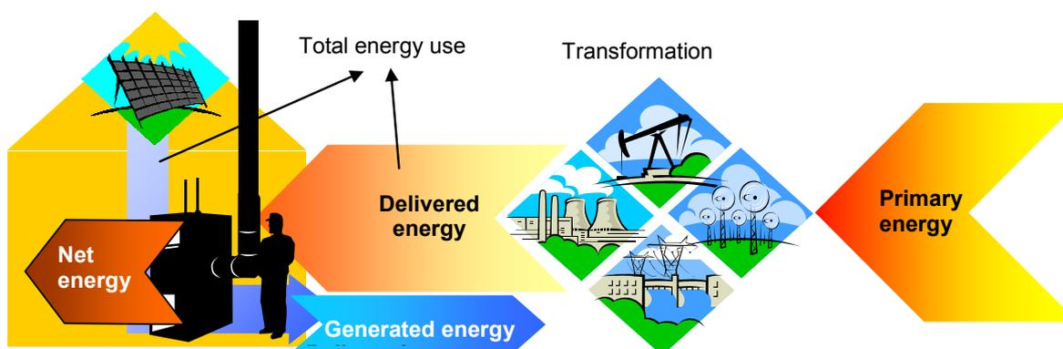
**Figure 1:** Energy flows to and from building: the primary energy vectors are transformed and transported to be delivered to the building in a useable form. In the building, the delivered energy is transformed into used energy, losses and possibly exported energy. The building may also have its own energy production from renewable energy sources.
