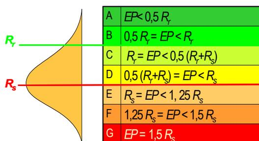
**Figure 4:** Proposal for sorting buildings given in prEN 15217. For each building type, the thresholds between classes are based on the average energy rating of the existing building stock,  $R_s$ , and on the national limit for new buildings,  $R_r$ . Like in other energy certification schemes, each class corresponds to a colour from green (A) to red (G).
