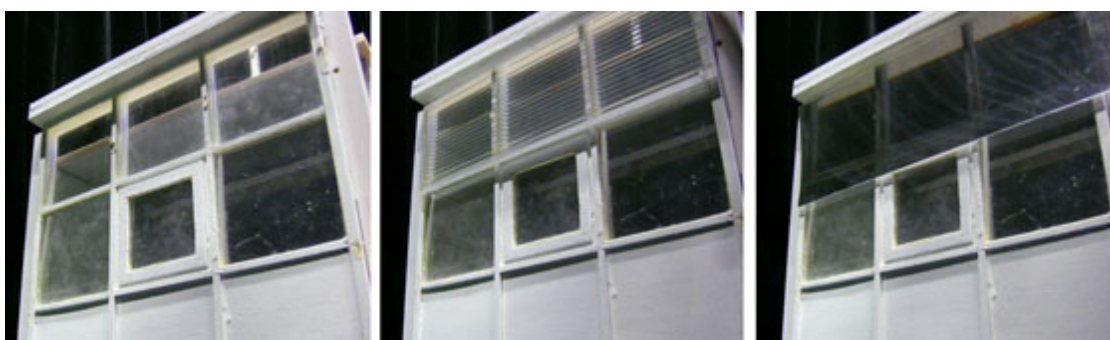
Figure 3: Glazing systems mock-up used on 1:10 scale model; (Left) 2mm.-single clear acrylic foil with neutral filter; (Middle) laser cut panel and (Right) 3M prismatic film.
