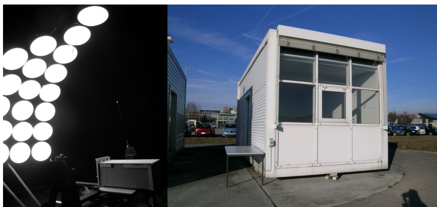
Figure 2: (Left) Scale model under scanning sky simulator; (Right) Full-scale test module on EPFL campus.
