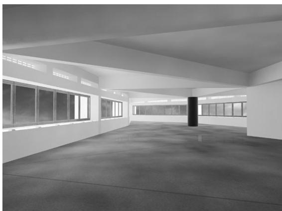
**Figure 4:** Computer daylight studies. On 21 June, the overhang and down-stand fascias cut out low angle sun.
