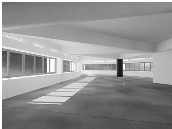
**Figure 5:** Computer daylight studies. The sunlight penetration at 3pm on 21 December.
