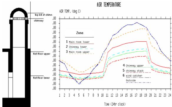
**Figure 5 :** Temperatures according to zones
