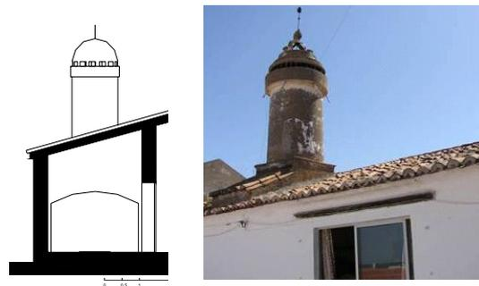
**Figure 1 and Figure 2:** Section of the adjacent room of chimney and photo of the exterior of the chimney
