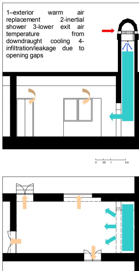
**Figure 3:** Section and Plan of the chimney and adjacent room (not on scale)
