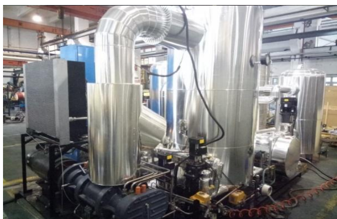
Figure 4: Water vapor compression heat pump.
