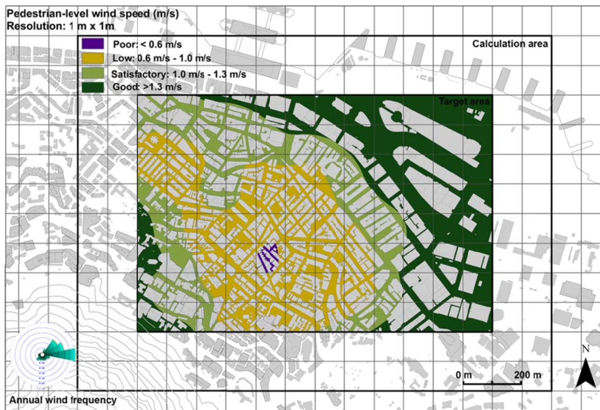
Figure 12: Pedestrian-level wind speed map, which was classified as Class 1 (Poor, <0.6 m/s), Class 2 (Low, 0.6 m/s -1.0 m/s), Class 3 (Satisfactory, 1.0–1.3 m/s), and Class 4 (Good, > 1.3 m/s).
