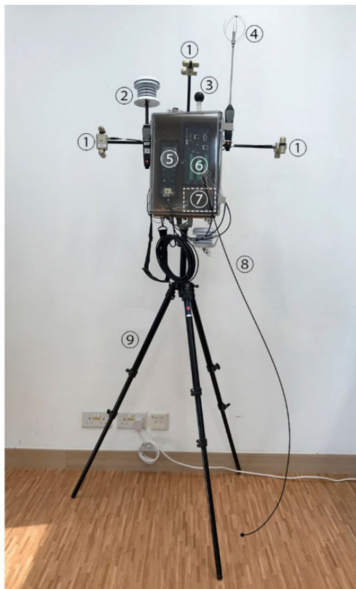
Figure 3. An example of the self-developed weather monitoring systems in the guideline.
