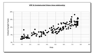
Figure 9 UVA of 160 low level windows, H is 3 times the base of the blocks
