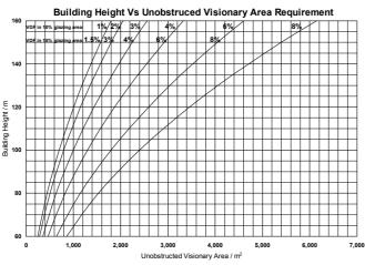
Figure 10 UVA requirement for different building height
