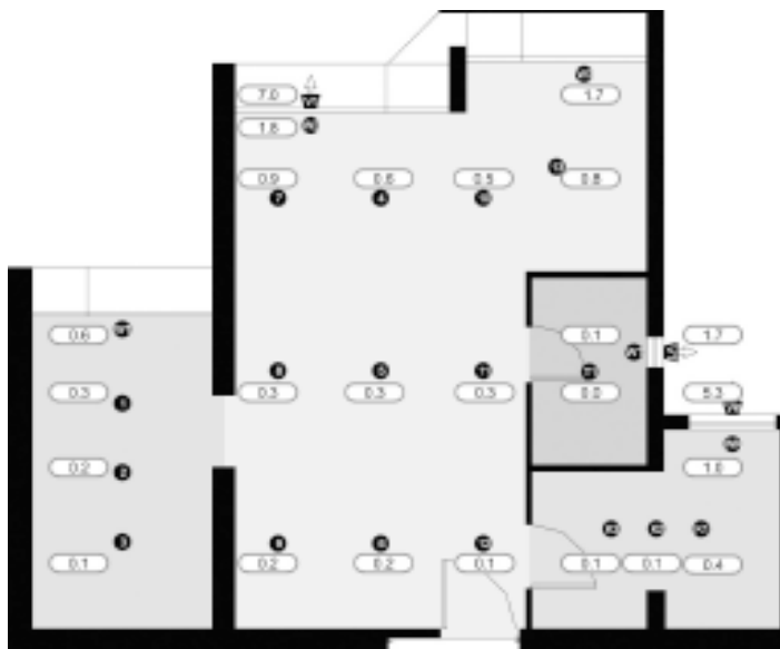
Figure 7: Daylight performance of a residential unit in high density sites in Hong Kong. Daylight Factor at the rear of the space is about 0.2%. The sensor V1 on the front face of the living room measures 7% VDF in this case. The sensor VK of kitchen window measures 5.3% VDF.
